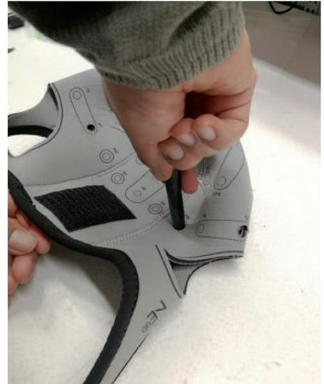
c. Pick a snap button of a color which corresponds to the channel's number.
