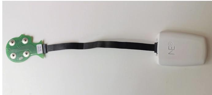
*Impedance troubleshooting.* Testboard allows to check the correct setup of the system when having high impedance values. Once you set up the testboard, in NIC, click on check impedances. If the values are correct, it means that the device works fine and the impedance issues are due to another component or the wrong setup. For further details about impedance check, please refer to NIC2 Instructions for Use.
